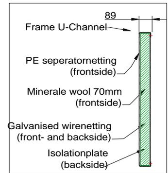
**Dimensions and pattern NOISEREDUCER® SA-80 Noise Barrier-A5:**
