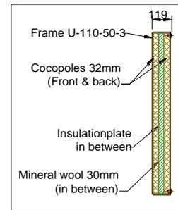
**Dimensions and pattern Kokowall DOUBLE ABSORPTION –A3 NOISE BARRIER**
